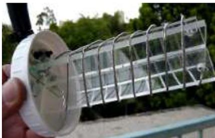
19. Now glue the electrodes wherever they touch the tower. A thin to moderate layer of GOOP is all it takes. A little 'bump' of Goop on every wire is more than enough to secure them in place.
