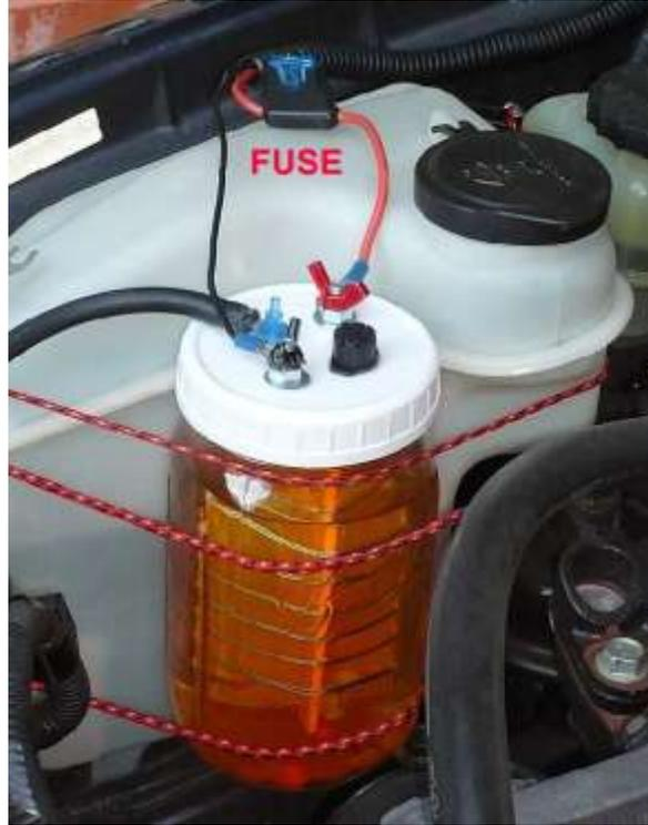
Fill the jar with DISTILLED WATER, leaving 1" of free space at the top. Add 1 teaspoon of Electrolyte (pure Baking Soda) and screw the jar onto the lid of the generator.
