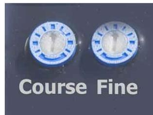
The way to set these is to set the fine pot at center, and then make your initial adjustments with the course pot only. Later, if you need to make small changes in the setting, you can do so with the fine pot.
